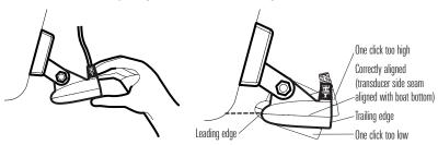
Adjust the transducer assembly vertically, until the seam on the leading edge of the transducer (the edge closest to the transom of the boat) is level and just slightly below the hull.
